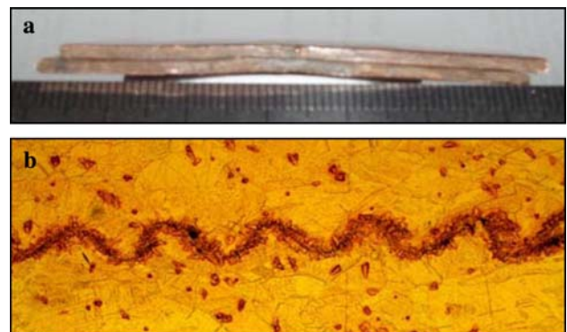
Fig. 5 (a) Copper plates welded by the water-projectile impact at the water velocity 1500 m/s and h = 3 mm. (b) Zoomed-in section of a micrograph of wavy interface of joined copper plates
