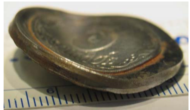
Fig. 16 General view of nickel alloy coin and steel plate welded by the water projectile impact at the water velocity 750 m/s (Exp. 14, Table 1)
