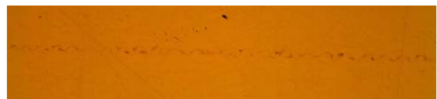
Fig. 6 Two copper plates welded by a water-projectile impact at the water velocity 1500 m/s and h = 3 mm. Notice uniformity of wavy seam along entire bond length (×100)
